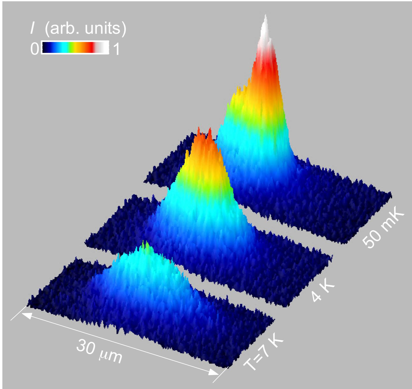
Sharp peak at trap center emerges with decreasing temperature
