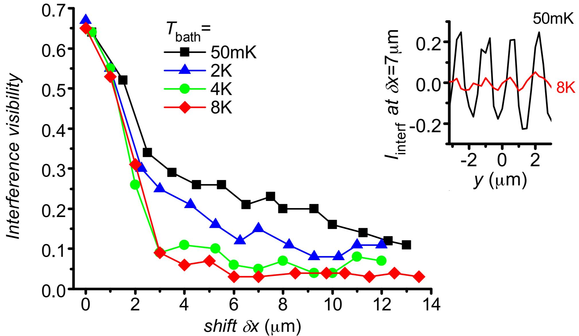
Coherence extends over entire cloud at  $T_{\text{bath}}=50\text{mK}$
